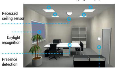
Modern lighting systems accesing to intelligent sensors and wireless technology. Controlling these lighting systems draws together the key aspects of flexibility and energy efficiency. A large number of parameters can be controlled conveniently via software: on/off/dimming, free control of light level, free control of light colour (with DT8), scene selections, group selections, individual addressing, timer, light control, motion detection, settings of basic DALI parameters.
